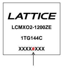
Numeric Character in fifth position of Datecode indicates Cu-wire material set Alpha Character in fifth position of Datecode indicates Au-wire material set
