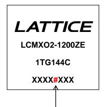
Numeric Character in fifth position of Datecode indicates Cu-wire material set Alpha Character in fifth position of Datecode indicates Au-wire material set
