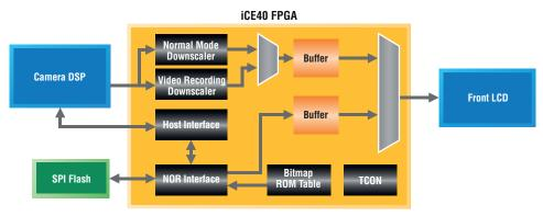
Figure 3: Using an iCE40 FPGA to implement front LCD integration and bitmap display.
