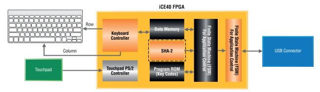
Figure 3: USB Docking Design using the iCE40 FPGA.
