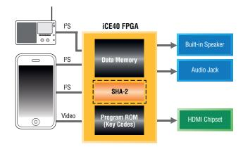
Figure 4: Media Docking Design using an iCE40 FPGA.
