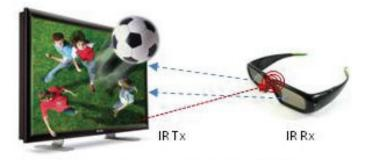
Figure 4: Shutter Glasses with 3D Display and IR
