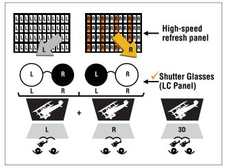
Figure 3: Shutter Glasses Operation Model
