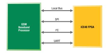
Figure 2: Examples of processor interfaces that can be used for interprocessor communication using the iCE40 FPGA.
