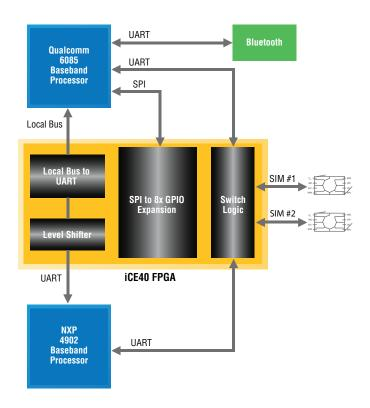
Figure 4: Interprocessor Communication Solution for Qualcomm 6085 and NXP 4902 Using the iCE40 FPGA.
