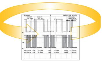
Figure 1: Auto-polling in a gyroscope sensor. Reading the same I<sup>2</sup>C transaction over time increases processor overhead.
