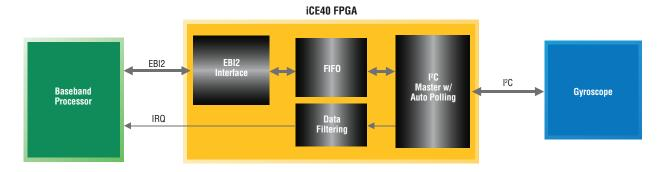
Figure 4: Auto-Polling implemented along with I<sup>2</sup>C Master to offload processor
