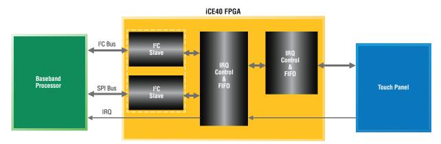
Figure 2: Interrupt Aggregator Design using the iCE40 FPGA
