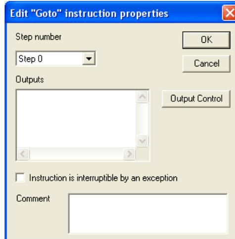
The target Goto step can be set using the Step number pull-down menu. You can set the outputs also along with this instruction.
