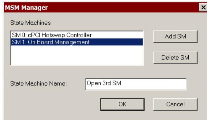
To add a state machine, selecting the place where you want to enter the next state machine, enter the name for the new state machine, and click **Add SM**. The window for sequence control will open. Note that the additional state machine has been created and opened for code edit. After the editing, the design can be recompiled and processed as discussed elsewhere in this manual.
