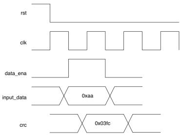
Before calculating the CRC code, the user can transpose the input data. For example, if the input data is 0x55 and the parameter INPUT\_DATA TRANSPOSE is set to '1', then this design uses data 0xAA to generate the CRC code.
