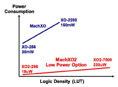
Figure 5: Static Power Comparison between MachXO2 and MachXO PLDs
