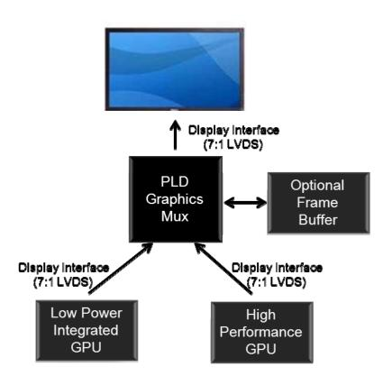
Figure 3: PLD-Based Graphics Multiplexer
