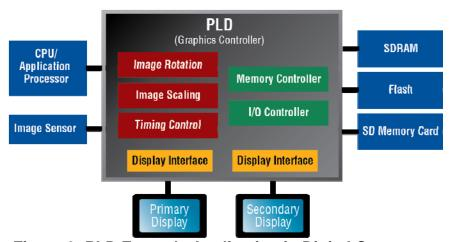
Figure 2: PLD Example Application in Digital Cameras
