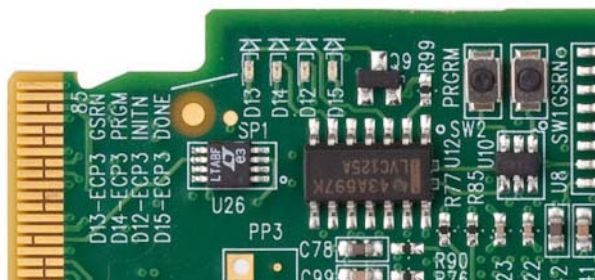
Figure 15. ECP3 Status LEDs and Pushbutton Controls (see Appendix D, Figure 30)
