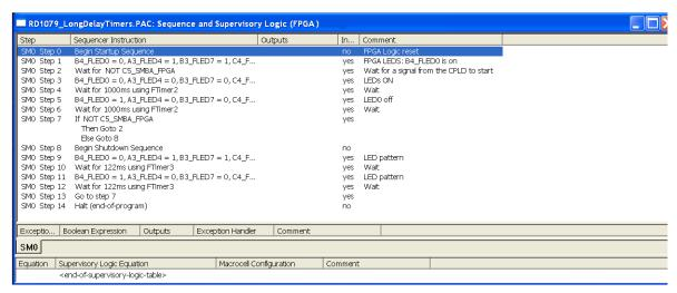
To edit the FTimer values, the user can simply double-click on the timer sequence step. The timeouts can be changed either before or after they have been added into a LogiBuilder sequence step.
