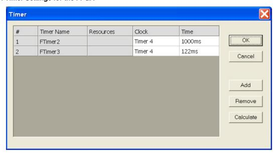
There is no pre-defined limit to the number of FTimers since these are built in the FPGA and are therefore LUT-based and dependent on the available FPGA LUT resources (as opposed to the CPLD section where timers are hardware-limited to three with a fourth used as a time-base for the FTimers in the FPGA).
