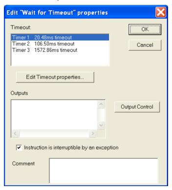
LogiBuilder can also be used to sequence outputs in the FPGA logic. A timer step is inserted in the sequence using the same method as for the CPLD, except when editing the properties, the FTimer dialog opens and allows multiple timers and values to be edited. The FTimer functional block allows the user to define timers from milliseconds to hours (see Figure 4).
