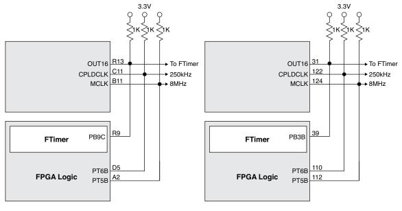
External Connections for 208-Ball ftBGA CPLD Logic and CLK Outputs
