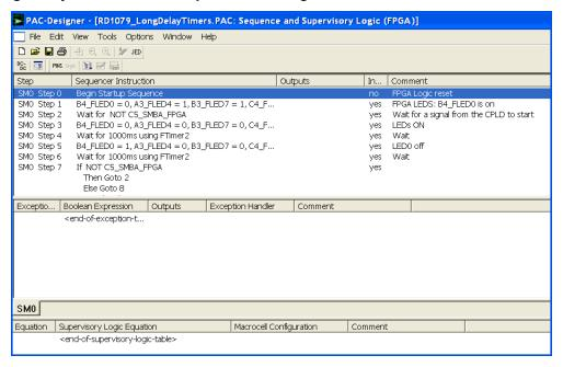
The user can easily edit any of the sequencer steps in the CPLD or the FPGA to experiment with I/Os, LCD, LEDs and push-buttons. Any timer delay in the CPLD or FPGA can be edited by simply clicking on the timer line in the code. Once an edit is made, compile the design and generate a JEDEC file for download.
