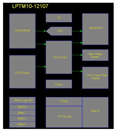
There is a functional block used for CTimers and another for FTimers. The Platform Manager CPLD section supports three timers that range from 32us to 1966ms. Simple pull-down menus allow the user to change all timer values that are available. To use a CPLD timer, a step is inserted in the LogiBuilder sequence with a "Wait For Timeout Value", as shown in Figure 2.
