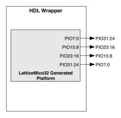
Placing the Verilog source code generated by LatticeMico32 System Builder into a Verilog or VHDL wrapper that swaps the byte lanes permits existing C/C++ firmware to continue to run without modification. It is also the less error prone technique for dealing with the change to the GPIO component.
