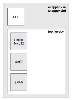
After restoring the PLL in the wrapper it is recommended that a circuit to manage *reset\_n* be implemented. LatticeMico32 platforms clocked by a PLL operate best when *reset\_n* is released after the PLL reports that it has locked to the input frequency. One possible solution is shown in Figure 7.
