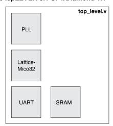
Figure 6 shows the structure of a LatticeMico32 platform after the PLL has been inserted according to the instructions provided above. The PLL is completely under your control. The clock source, feedback paths, and the various
