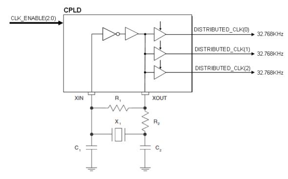
Figure 2 - CPLD with Crystal Pierce Circuit
