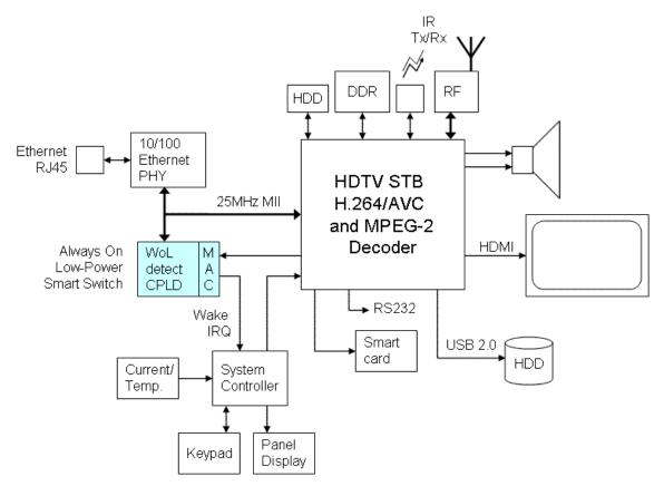
Figure 1 - IP-TV STB with CPLD-based Smart Switch
