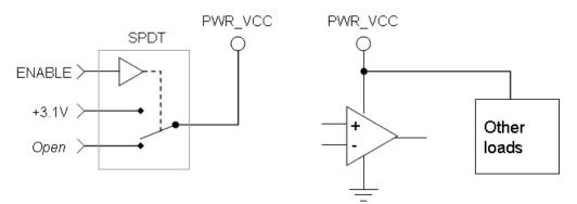
Figure 3 - Gating of On-Board Power Rails
