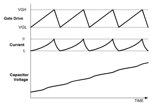
Figure 3 – Hysteretic current limiting cyclically allows MOSFET current to increase to a maximum allowable level, and then throttles it back to a slightly lower level. This technique provides many of the advantages of linear current control while sidestepping many of the potential stability issues.
