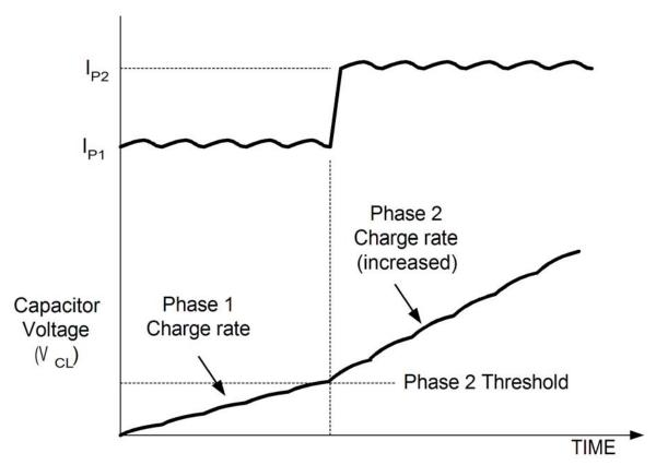
**Figure 4** – A two-phase switching strategy first charges the on-board capacitors at a low current when the switch MOSFET is subject to a high  $V_{DS}$ , and then increases the current when the capacitors are partially charged and the MOSFET experiences lower  $V_{DS}$ .
