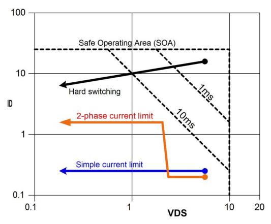
**Figure 2** – The Safe Operating Area (SOA) chart for a MOSFET shows the device's safe endurance limits for combinations of drain-to-source voltage and drain current. Different control strategies can be used to avoid excessively stressing the MOSFET when used as a hot swap load switch.
