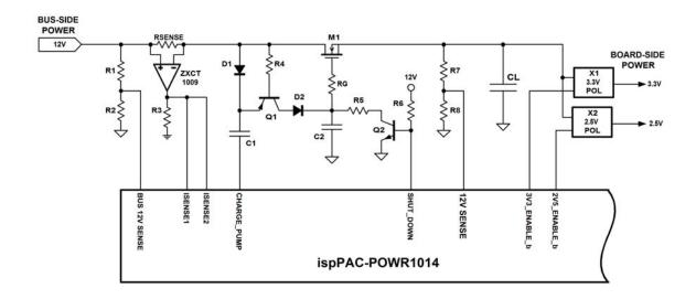
**Figure 1** – A hot swap controller typically employs a power MOSFET (M1) to connect the bus power to the internal board power systems after the board has been positively seated in its socket. Lattice's ispPAC-POWR1014 provides intelligent control that can be tailored to the application's requirements through its programmable logic and analog functions.
