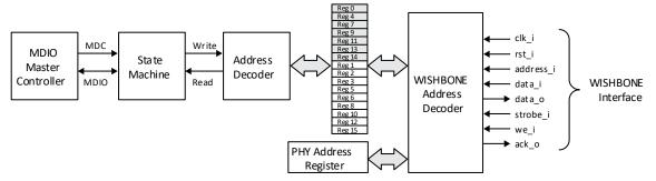
Figure 4.1. Block Diagram
