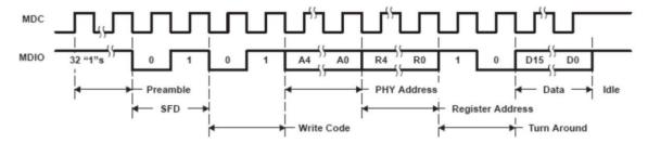
Figure 3.2. Write Timing
