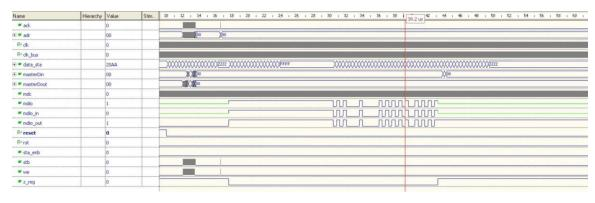
Figure 5.1. Write Operation (phy\_address=5'd1, reg\_address =5'd0 and data =16'hAA55)
