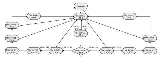
Figure 4.2. Read/Write State Machine
