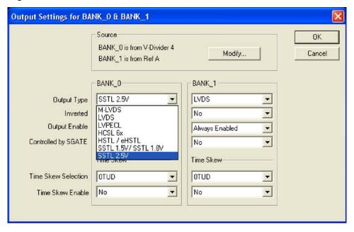
The external PLL feedback is used here to generate zero-delay clock output. Users can make use of the phase and time delay adjustment in the device to further compensate for the board routing delay. The phase skew adjustment can be modified in the Phase Skew Manager block in PAC-Designer. The time skew can be modified in the output block as shown in Figure 2.
