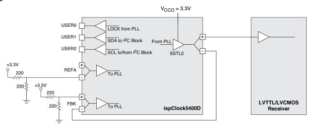
Conceptually, the SSTL and LVCMOS drivers are equivalent since both consist of a pull-up PMOS and pull-down NMOS. The difference in the driver behavior is determined by the off-chip termination circuitry. The LVTTL/LVC-MOS input and output specifications are defined in JESD8C, the JEDEC standard for Nominal 3.0V/3.3V Supply
