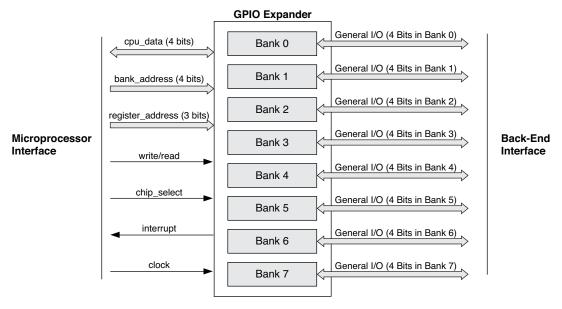
Note: The cpu\_data width and general I/O width can be configured by the designer. The default value is 4.
