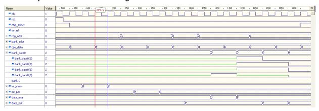
Figure 9 shows the timing of the read operation of the registers in bank 0.
