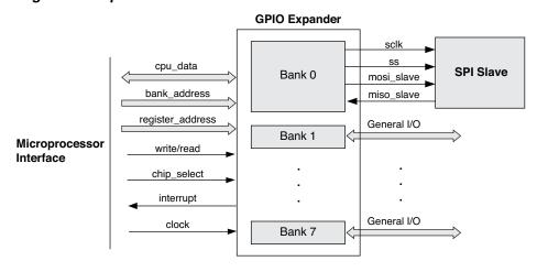
This example selects bank 0 of the GPIO Expander to connect with the SPI slave device. Three general I/O ports in bank 0 are configured as outputs by the microprocessor and are used as the serial clock signal, slave select signal and master-out-slave-in signal respectively, as defined by the SPI protocol. The last port in bank 0 is configured as an input by the microprocessor and is used as the master-in-slave-out signal.
