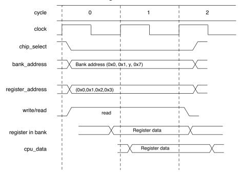
Figure 6. Microprocessor Reads Data from the Register
