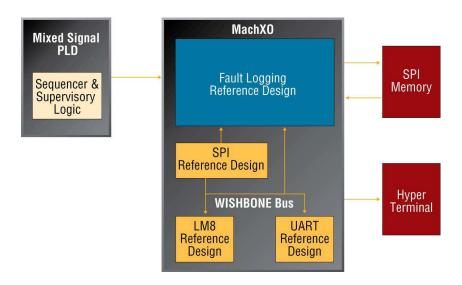
Figure 2 – Using MachXO PLD for Logging Environmental Data
