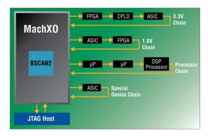
Figure 3 – Using MachXO PLD to Break Up Long JTAG Chains
