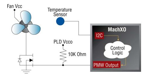
Figure 1 – Fan Control Using MachXO PLD
