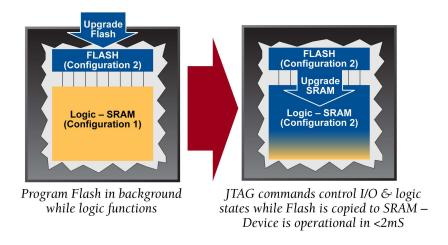
Figure 5 - TransFR operation using MachXO PLDs
