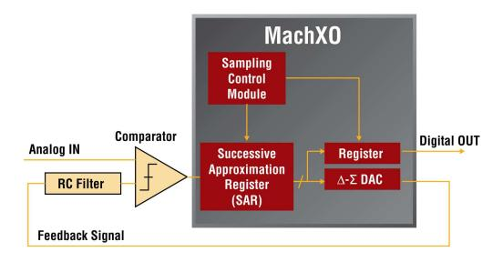
Figure 4 – Voltage Monitoring Using MachXO and Delta Sigma ADC implementation
