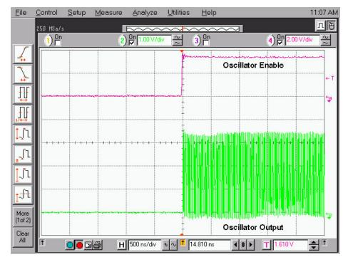
Figure 3. Initial Transitions of Enabled Oscillator
