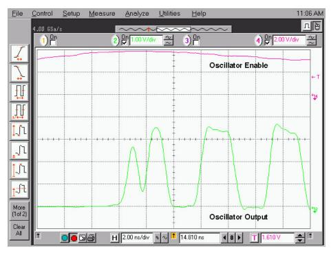
In this case where the reference oscillator is gated on, either by the output enable pin of the oscillator or by other means of asynchronous enable, the RESET pin should be activated after the reference has been enabled and the clock input to the ispClock is stable.
