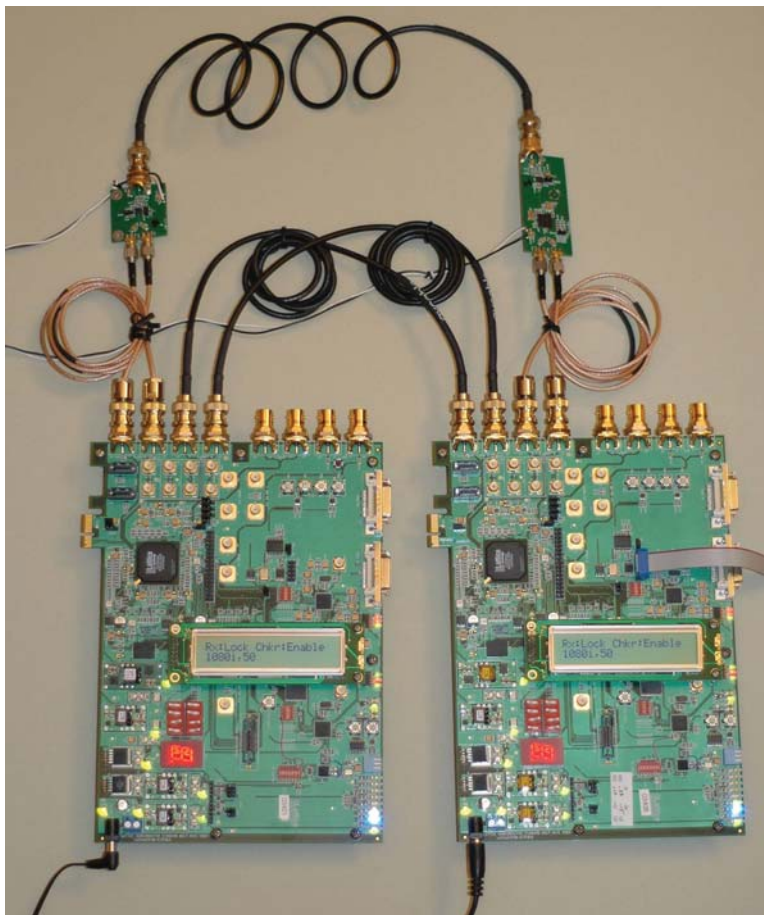
Figure 22. Connection Example 1 Using Two SMPTE SDI Boards
