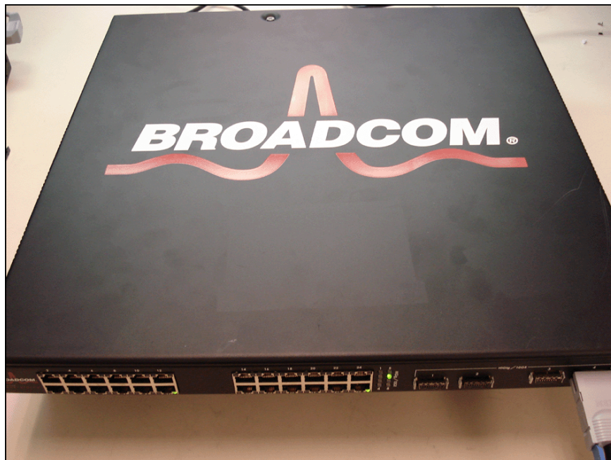
Figure 2. Broadcom BCM56580 Network Switch
