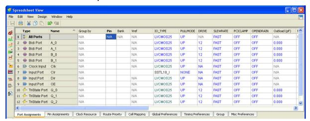
Figure 8-4. Port Attributes Tab of Spreadsheet View
