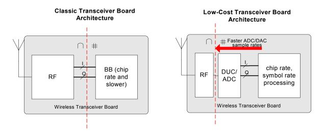
Figure 9- Wireless Transceiver Board Architectures
