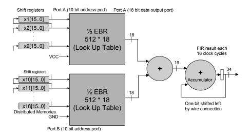
Figure 3 - Use of Lattice Block Memories as FIR Multipliers
