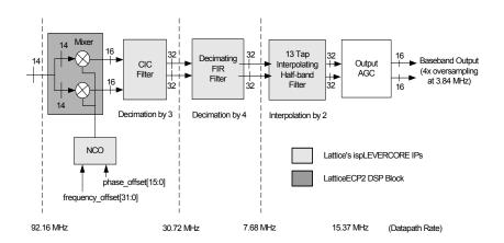
Figure 8 - Digital Down-Converter for WCDMA Application
