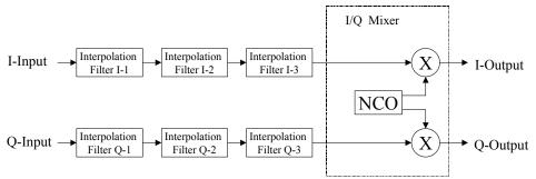
Figure 2 - DUC Structure
