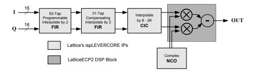
Figure 7 - Digital Up-Converter for Digital Radio Application
