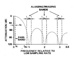
Figure 6 - Frequency Response for a CIC Filter
