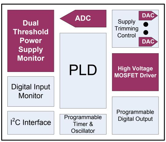
FIGURE 2 - Power Manager Block Diagram
