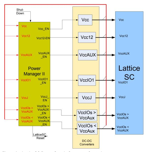
Figure 3 – LatticeSC Power Supply Sequence Control
