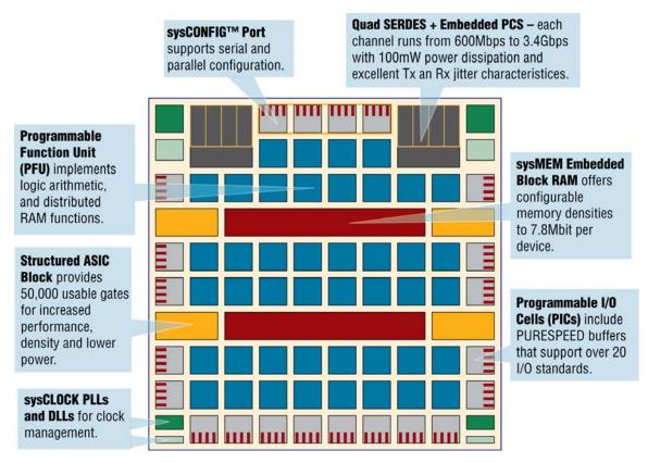
Figure 1 – LatticeSC Block Diagram
