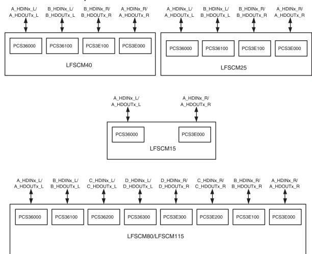
The user must make note that all flexiPCS/SERDES quads are not bonded out to pins on the selected package. Verify in the package listing that the HDIN and HDOUT pins are available for the selected quad before selecting the location.
