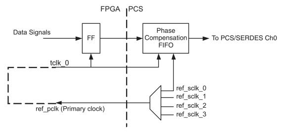
The ref\_pclk output clock is derived from the reference clock. There is a mux controlled via a memory map register which controls the source of this clock based on channel. This mux is useful if a transmit channel is powered down and needs to switch to another channel.
