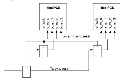
By using a local flip-flop to drive each flexiPCS's transmit reset lines the resets will be balanced to the tolerance of the primary clock (~100ps across the device).
