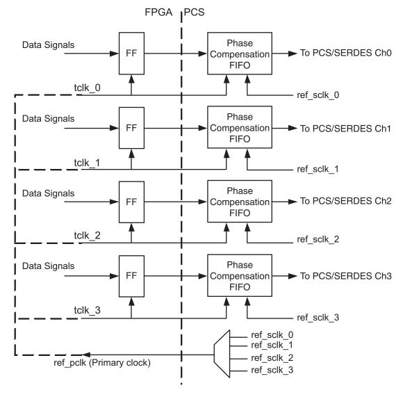
Figure 5. flexiPCS Interface Transmit Clocking for all Four Channels
