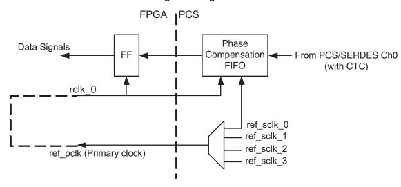
The CTC block is written to using the recovered clock derived from received data. The CTC block is read using the local reference clock which is the transmit clock. Since the CTC is read using the transmit clock the receive interface is the exact same as the transmit interface when using the CTC.
