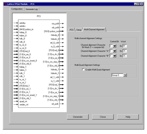
Figure 3. IPexpress flexiPCS Module Multi-Channel Alignment Tab
