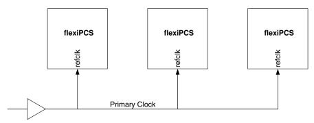
The designer can choose to use the FPGA source reference clock when creating the flexiPCS module in IPexpress. To force the usage of a primary clock, use the USE PRIMARY NET preference on the FPGA sourced reference clock net.
