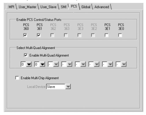
Only flexiPCS quads that are available on the device are allowed to be selected. Once a flexiPCS location is selected a flexiPCS specific port will exist for the particular flexiPCS quad. For example, PCS360 has dedicated ports on the system bus named pcs360\_in[16:0] and pcs360\_out[44:0]. Likewise the flexiPCS has ports sysbus in[44:0] and sysbus out[16:0] that connect to these system bus ports.
