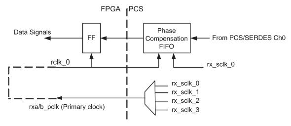
Figure 10. flexiPCS Interface Receive Clocking Using Secondary Output Recovered Clock
