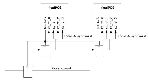
By using a local flip-flop to drive each flexiPCS's receive reset lines the resets will be balanced to the tolerance of the primary clock (~100ps across the device).
