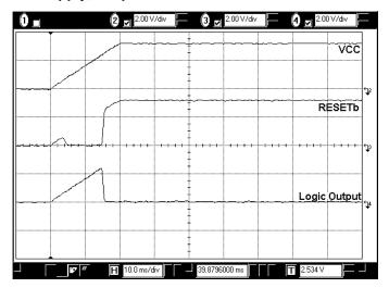
Figure 23-3. Startup with Slow Supply; Output Resets High
