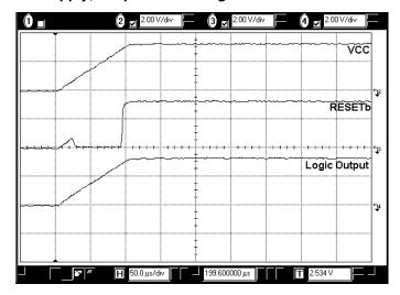
HVOUT pins that have been programmed for charge pump operation pull down during power-on reset regardless of the reset levels programmed into their associated macrocells. This is a safety feature that ensures that the external MOSFETs that these pins control will be off when the ispPAC-POWR1014/A begins its power supply sequencing operations.
