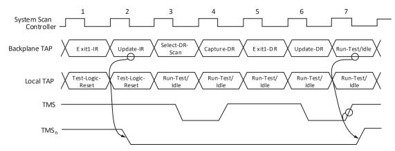
Figure 8.1. Local Scan Port Synchronization on Second Pass
