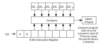
Figure 6.1. Direct Addressing: Device Address Loaded into Instruction Register
