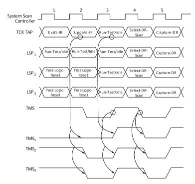
Figure 8.2. Synchronization of the Three Local Scan Ports (LSP<sub>1</sub>, LSP<sub>2</sub> and LSP<sub>3</sub>)
