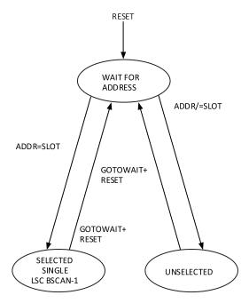
Figure 2.3. Selection Controller State Machine
