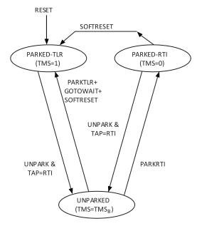
Figure 2.4. Local Port Configuration State Machine
