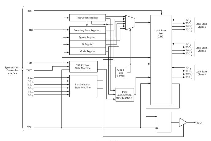
Figure 1.1. BSCAN1 Block Diagram
