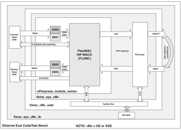
Figure 2 shows the LatticeSCM Ethernet flexiMAC core in a system context with other IP (e.g. PCS, System Bus-LatticeSCM hard IP) and user defined soft logic (e.g. client and Statistics logic). There are different levels depicted in the figure:
