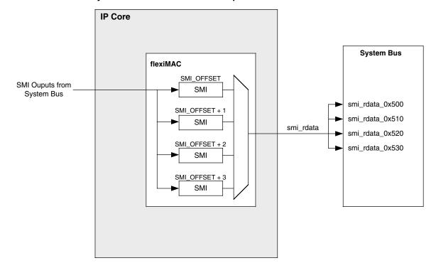
Figure 12. flexiMAC and System Bus Connections Example
