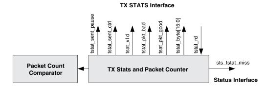
Pause frame transmission is indicated by tstat\_sent\_pause and tstat\_sent\_ctrl signals.
