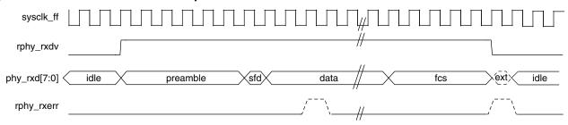
sysclk\_ff: provides the timing reference for the rphy\_rxdv, rphy\_rxd and rphy\_rxerr signals.
