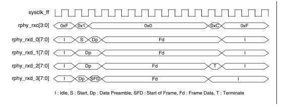
**sysclk\_ff:** provides the timing reference for the transfer of the rphy\_rxc[3:0] and rphy\_rxd\_[0:3] [7:0] signals from typically the PCS.
