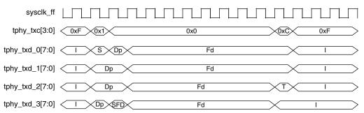
I: Idle, S: Start, Dp: Data Preamble, SFD: Start of Frame, Fd: Frame Data, T: Terminate
