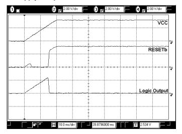
Figure 7-3. Startup with Slow Supply; Output Resets High
