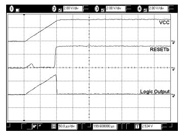
Figure 7-5. Startup with Fast Supply; Output Resets High
