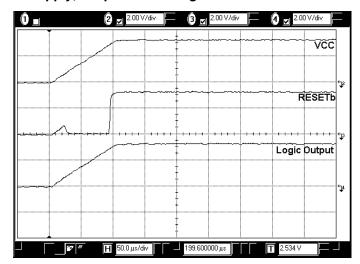
HVOUT pins that have been programmed for charge pump operation pull down during power-on reset regardless of the reset levels programmed into their associated macrocells. This is a safety feature that ensures that the external MOSFETs that these pins control will be off when the ispPAC-POWR1220AT8 begins its power supply sequencing operations.
