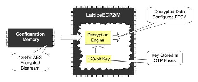
Figure 6 -- Bitstream Encryption Deters Design Piracy
