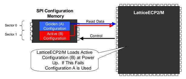
Figure 5 -- Using Dual Boot Configuration With Dual Boot
