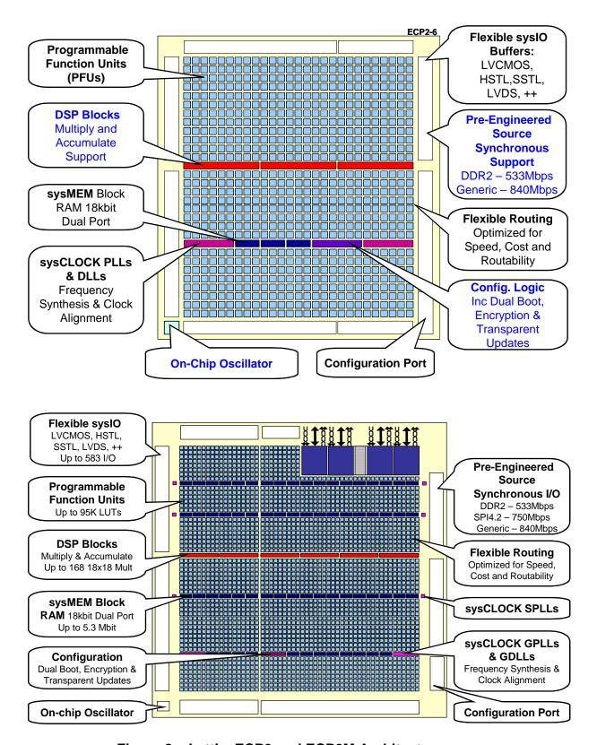
Figure 2 – LatticeECP2 and ECP2M Architectures
