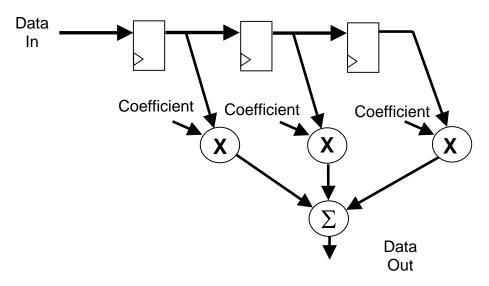
Typical Finite Impulse Response FIR Filter
