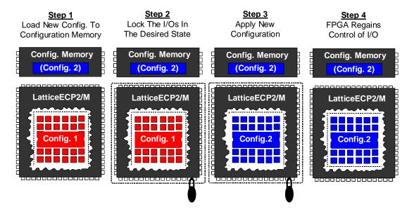
Figure 7 -- TransFR I/O Allows FPGA Update While Equipment Operates
