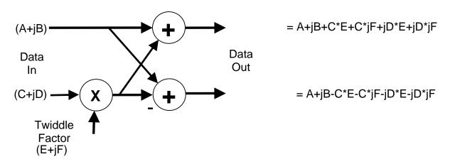
Radix-2 Butterfly Element Commonly Used In Fast Fourier Transformation
