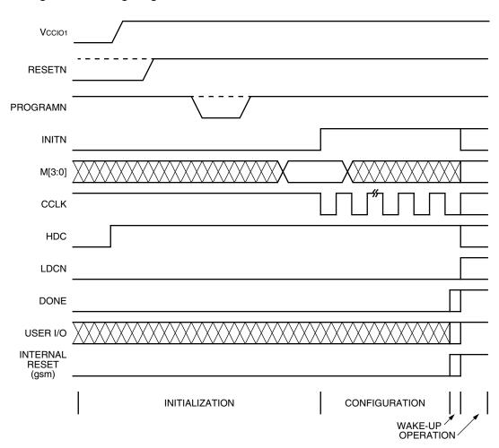
Figure 26. Configuration Timing Diagram
