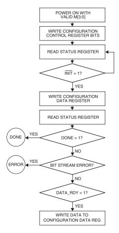
In general, a PROM image of the configuration bitstream is generated in EXO (S-record) or MCS (Intel\*) format and linked into the firmware image during the compilation process. PROM images can be created using Lattice ispVM® software. At power-up, the LatticeSC device examines the MODE pins, activates the MPI in 8, 16, or 32-bit interfaces and waits for firmware to control and write the configuration data into the device.
