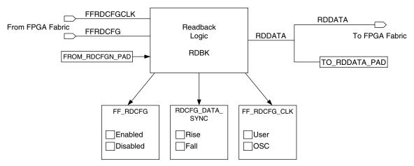
The library element connects to the user design via a three-port interface. The interface uses these connections to control and manage the readback of the bitstream data. The data read is available to be routed to the FPGA fabric. The data is clocked by a user-supplied clock or the on-chip oscillator. The maximum readback is 150MHz.
