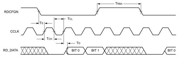
The RDCFGN input pin is also used to control the global tri-state (TSALL) function. Before and during configuration, the TSALL signal is always driven by the RDCFGN input and read back is disabled. After configuration, the selection as to whether this input drives the readback or global tri-state function is determined by a set of bitstream options. If used as the RDCFGN input for readback, the internal TSALL input can connect internally to be driven by any input pin.
