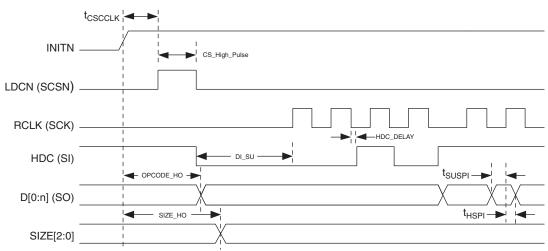
Figure 16. SPI Programming Timing Waveform
