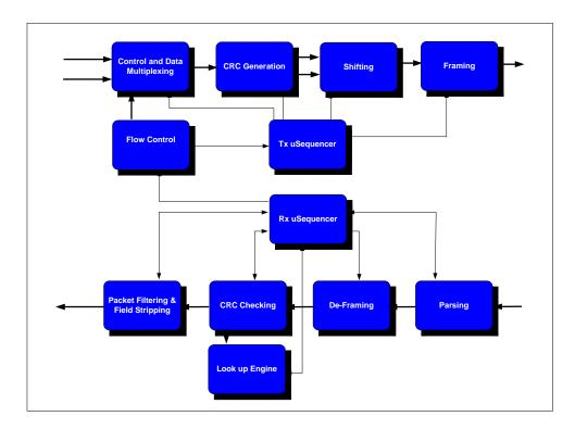
Figure 2 - flexiMAC Architecture
