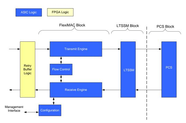
Figure 5 – PCI Express Data Link Layer + PCS Partitioning
