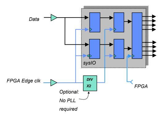
LatticeSC PURESPEED I/O DDR Input
