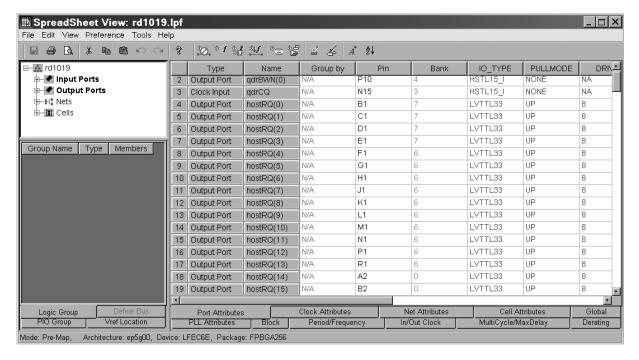
The Design Planner produces a comma-separated-value (CSV) report file of all physical device pins and logic details.
