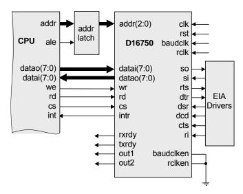
Typical D16750 and processor connection is shown in figure above.
