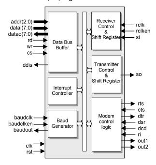
Receiver Control - Receiving starts when the falling edge on Serial Input (SI) during IDLE State is detected. After starting the SI input is sampled every 16 internal baud cycles as it is shown in figure below. When the logic 1 state is detected during START bit it means that the False Start bit was detected and receiver back to the IDLE state.
