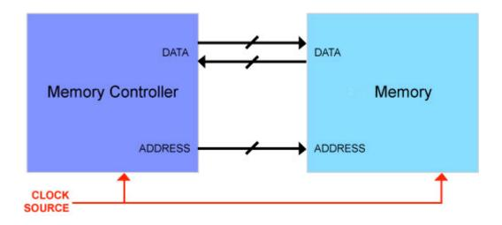
Figure 2 - Typical Non-DDR System
