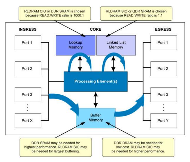
Figure 1 - Memories in Networking: Different Functions Require Different Approaches
