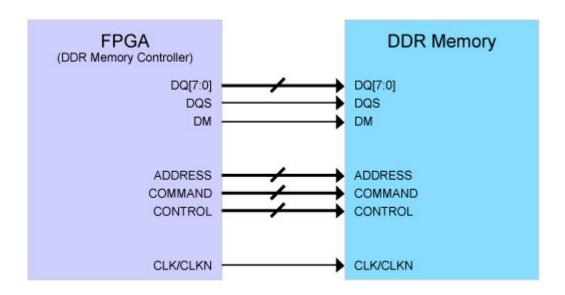
Figure 3 - Typical DDR interface
