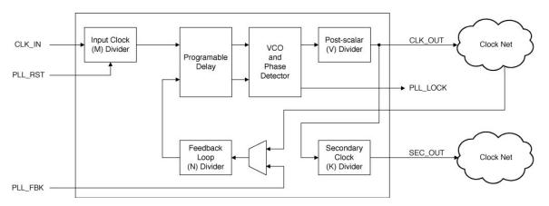
The ispXPLD 5000MX devices provide two PLL circuits. The optional outputs CLK\_OUT can be routed to an I/O pin. The optional PLL\_LOCK output is routed into the GRP. The optional PLL\_FBK into can be routed directly from a pin. Figure 6 shows the ispXPLD 5000MX PLL block diagram.
