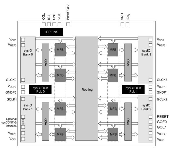
The MFB consists of a multi-function array and associated routing. Depending on the chosen functions, a single multifunction array uses up to 68 inputs from the GRP and the four global clock and reset signals. The array outputs data along with certain control functions to the macrocells. Output signals can be routed internally for use elsewhere in the device and to the sysIO banks for output. The various configurations are described in more detail in the following sections.
