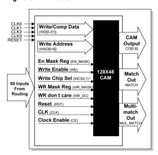
To further enhance the flexibility of the CAM a mask register is available. If enabled during updates, bits corresponding with those set to 1 in the mask register are not updated. If enabled during compare operations, bits corresponding to those set to 1 in the mask register are not included in the compare. A write don't care signal allows don't cares to be programmed into the CAM if desired. Like other write operations the mask register controls this.
