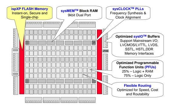
Figure 2 – LatticeXP Architecture
