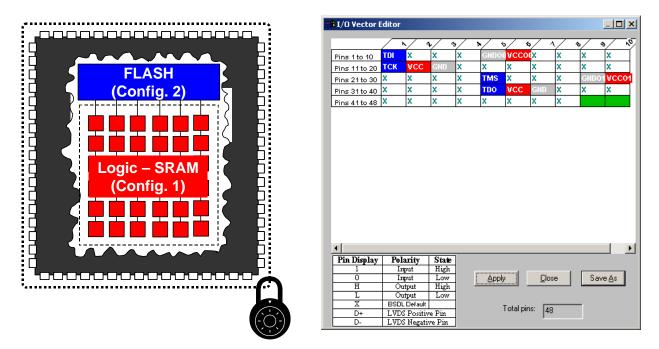
Figure 5 -- Locking I/O States Using ispVM
