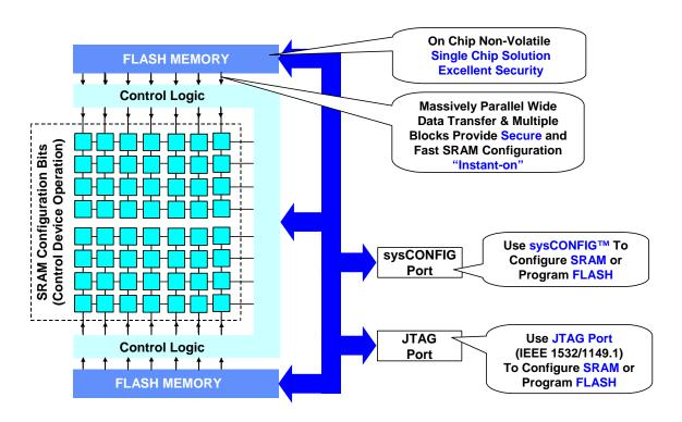
Figure 3 – Configuration Memories in the LatticeXP
