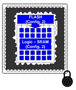
Figure 6 -- Updating the SRAM Configuration From FLASH
