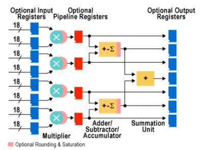
These blocks are able to perform all functions at a speed of 250 MHz, resulting in overall processing capacity of 10,000 MMACs (Mega Multiply Accumulate operations). As the data for processing is presented to these sysDSP blocks completely by hardware (as opposed to a microprocessor fetching the data from its memory), the performance of these blocks is close to benchmark-based expectations. The pipeline registers enable DSP processing operations at peak
