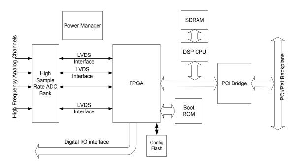
DSP Board With Integrated 4 Channel Data Acquisition With Playback
