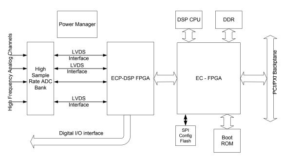
Proposed Architecture: 40 MSample DSP Board With Integrated 4/8 Channel Data Acquisition With Playback & Control
