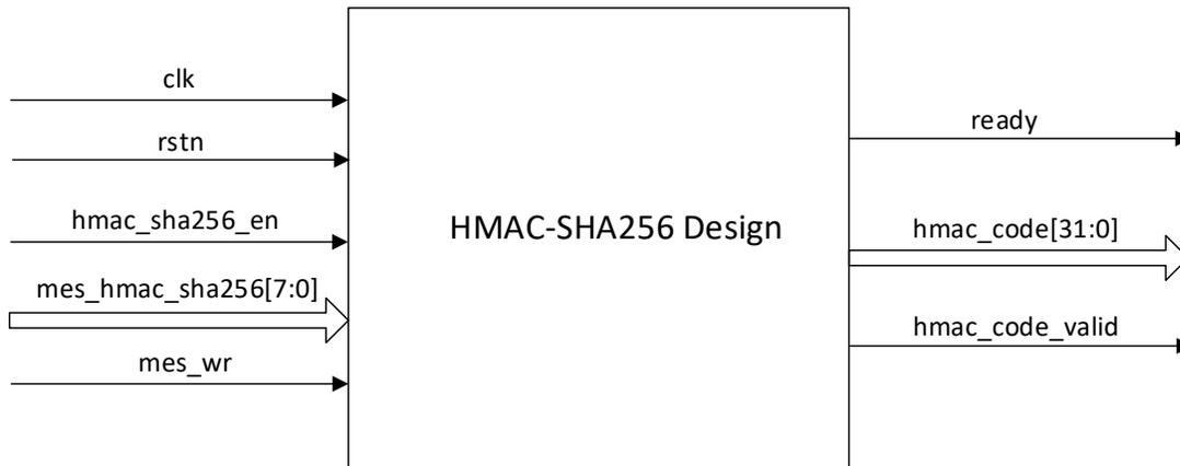
**Figure 4.1. I/O Diagram of the HMAC-SHA256 Design**
