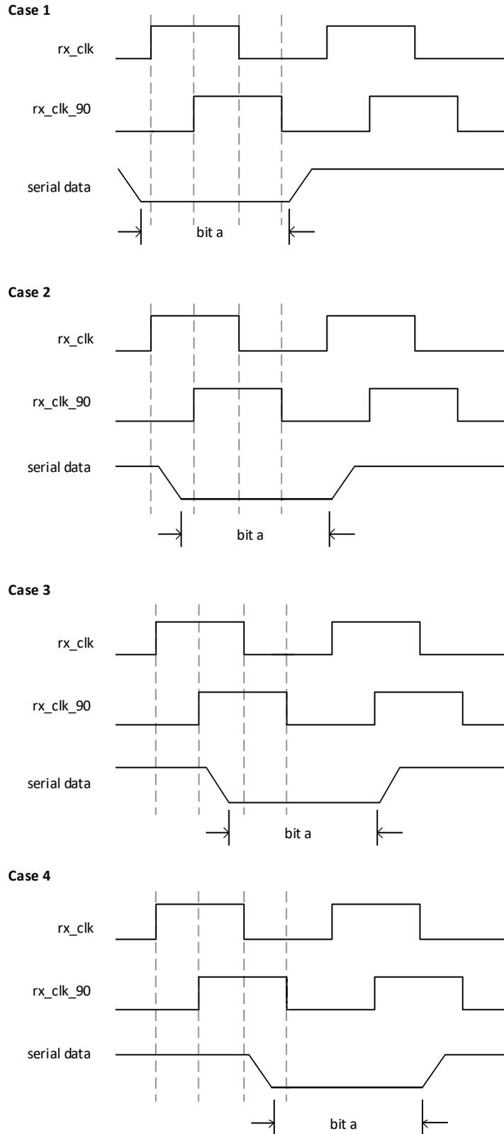
**Figure 7.1. Oversampling Data Using Different Clock Edges**
