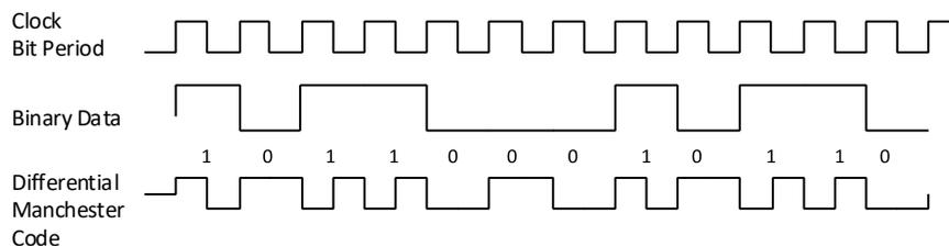
**Figure 6.1. Example of Differential Manchester Encoding**
