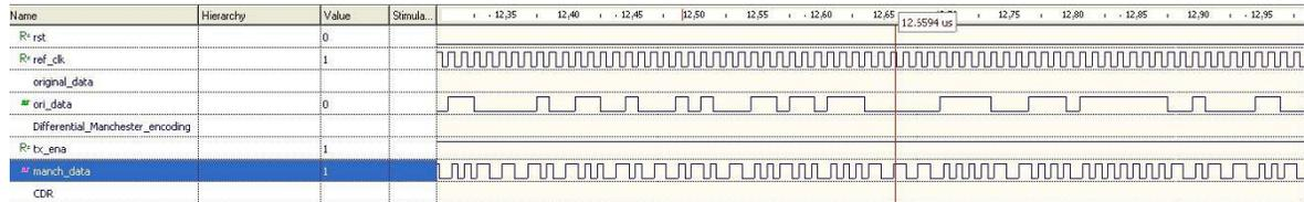
Figure 9.1. Differential Manchester Encoding
