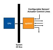
The ispGDXV provides an in-system programmable signal routing device for industrial control and instrumentation applications.
