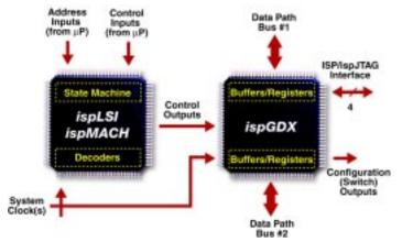
ispGDXV devices are the perfect complement to Lattice ispLSI® and ispMACH™ devices. Use ispLSI and ispMACH devices for fast control logic and ispGDXV devices for fast datapath logic.
