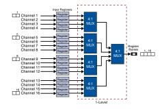
Multiplex 16 slow-speed channels into a single highspeed channel.
