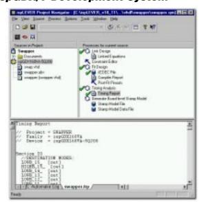
The ispLEVER Development System supports ispGDXV and ispGDX design entry, timing analysis, programming and timing simulation interfaces using a simple language syntax and an easy-to-use graphical user interface. The software runs under Windows® XP, Windows 2000, Windows 98 and Windows NT®. A command line driven version is also available to run on Sun Solaris and HP-Unix workstations.
