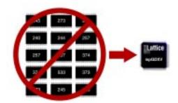
The ispGDXV replaces dozens of discrete interface devices, reducing PCB area and switching noise.
