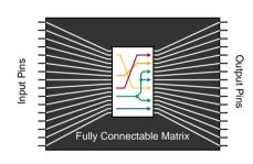
The ispGDX Global Routing Pool (GRP) is an in-system programmable wide signal switching matrix.
