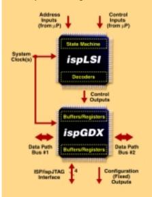
ispGDX devices are the perfect complement to Lattice ispLSI. Use ispLSI devices for fast Control Logic and ispGDX devices for fast Datapath Logic.
