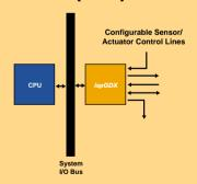
The ispGDX provides an in-system programmable signal routing device for industrial control and instrumentation applications.
