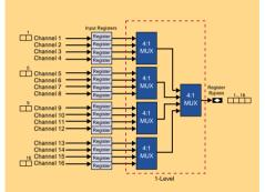
Multiplex 16 slow-speed channels into a single high-speed channel.
