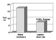
Figure 7: 8-Bit Parity Generator
