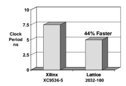
From a data sheet perspective, one would expect these devices to operate at roughly the same performance levels, however, actual implementation of 3 common benchmark functions (16-bit Bus Data Path, 8-bit Parity Generator and a Divide-by-2 Clock Divider) shows Lattice to be anywhere from 44% to 133% faster than Xilinx. The results of these three performance benchmarks are shown in figures 6, 7 and 8 above.
