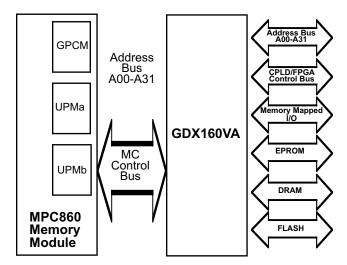
Figure 2. CPM/GDX160VA Block Diagram
