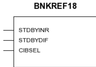
Figure 2.2. Primitive for Bank Controller
