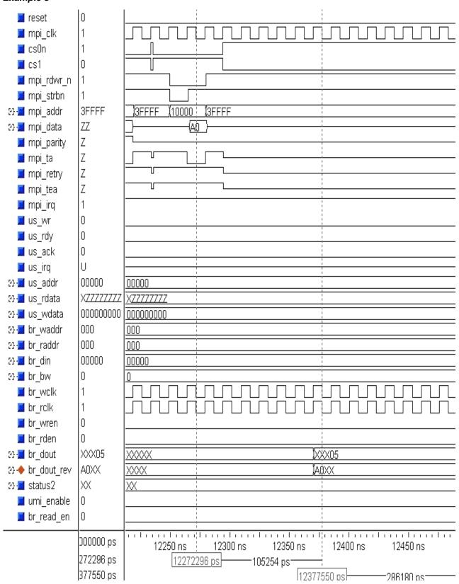
Figure 52. Functional Simulation Waveform for the MPI Write Transaction at Address 0x08001 with Data AA, in Example 3
