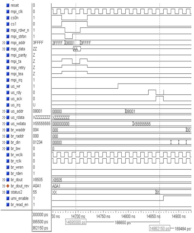
Figure 53. Functional Simulation Waveform for Read Transactions of the System Bus Block RAM with the FPGA Logic, in Example 3
