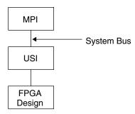
First the designer needs to create the system bus module in HDL. This is done using the ispLEVER Module/IP Manager Wizard.
