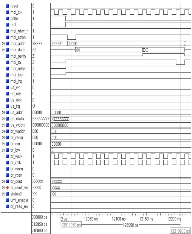
Figure 51. Functional Simulation Waveform for the MPI Write Transaction at Address 0x10000 with Data A0, in Example 3
