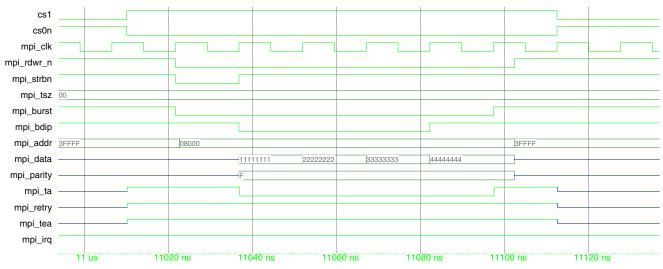
Figure 7. MPI Burst Write Transfer Timing
