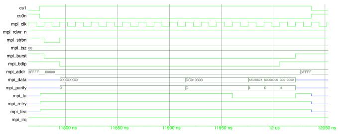
Figure 8. MPI Burst Read Transfer Timing
