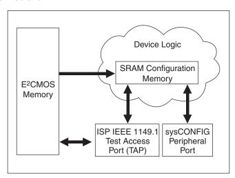
In this Usage Guide the terms "configuration" and "programming" are both used. "Configuration" is the act of downloading information into the SRAM memory while "programming" is the act of loading and storing data in the E<sup>2</sup>CMOS memory.
