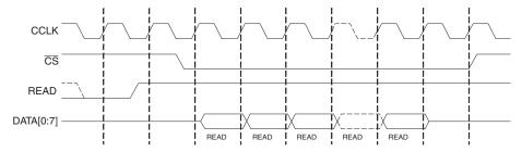
Figure 6. ispXP Read Cycle Flow Diagram
