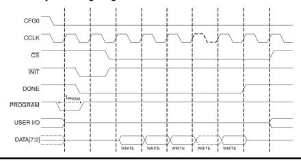
Figure 4. Synchronous Write to Configuration SRAM Flow Diagram
