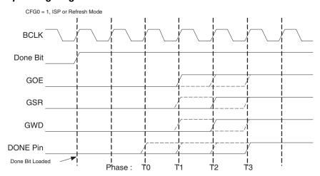
Figure 9. sysCONFIG Wake-up Timing Diagram
